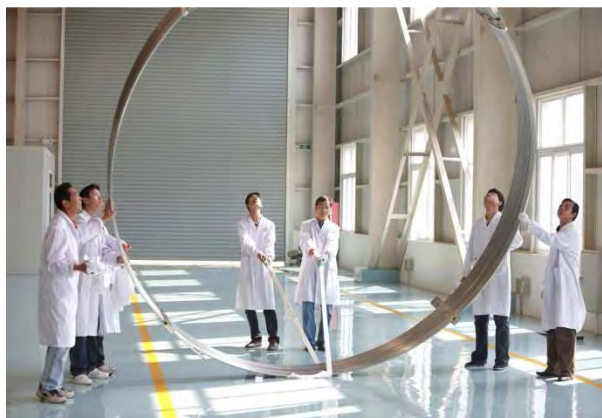
FIG. B-2. Hoisting superconducting correction coils to be used in ITER, Institute of Plasma Physics, Hefei, China.
