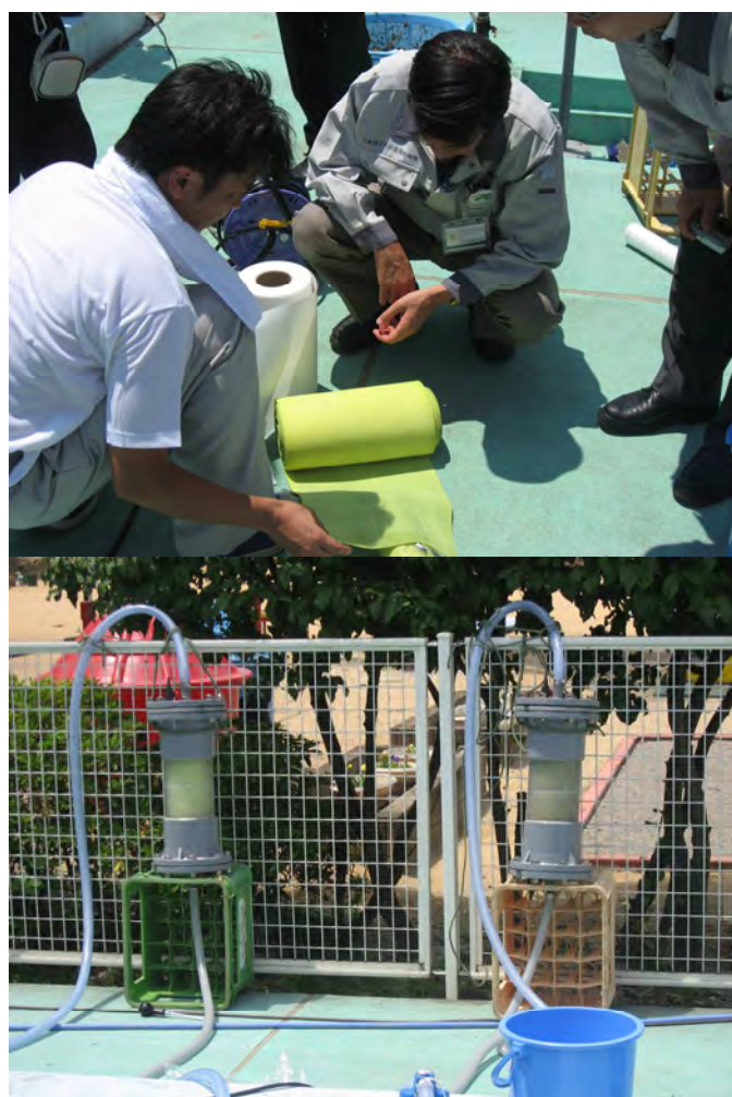
FIG. H.1. Grafted membranes being used for removing radiocaesium from water in the Fukushima area (courtesy of JAEA Takasaki, Japan).
