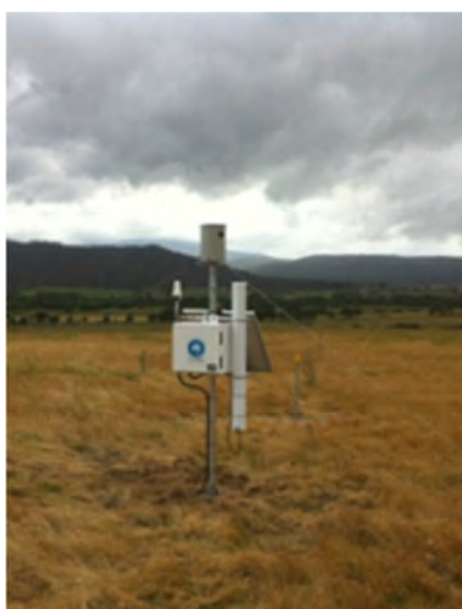
FIG. D.1. COSMOS installation in a grazed pasture in Australia (photo courtesy of Dr Chris Smith, Commonwealth Scientific and Industrial Research Organization (CSIRO): Land and Water, Canberra).
