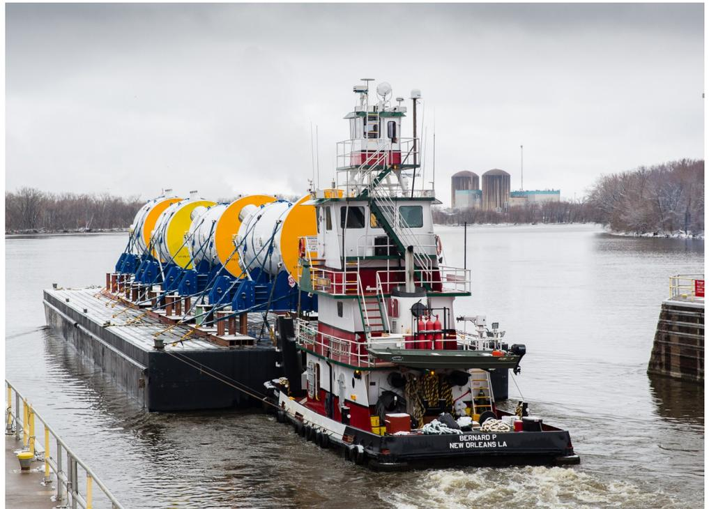
*Replacement steam generators for unit 2 of Xcel Energy’s Prairie Island nuclear energy facility pass through a lock near Red Wing, Minn. The plant is in the background. For a video clip, see [here](#). (Photo credit: Xcel Energy)*
